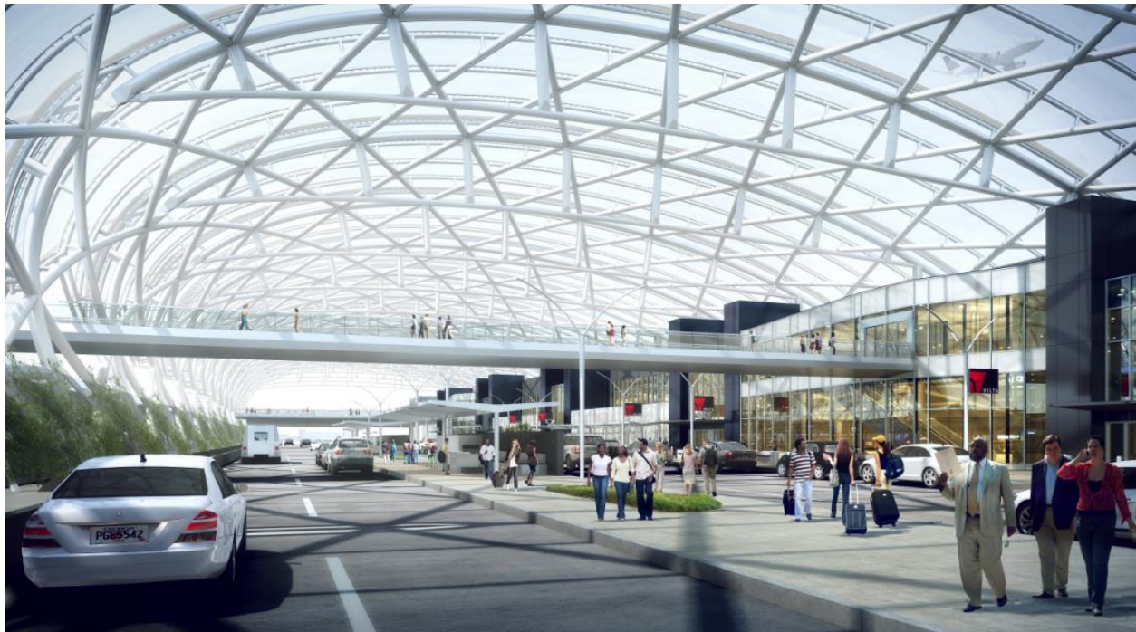
Figure 4: A new vision for the landside approach to the domestic terminal, with a canopy covered in transparent ETFE paneling, pedestrian walkways spanning the traffic lanes, and a new terminal facade. Rendering: HOK
